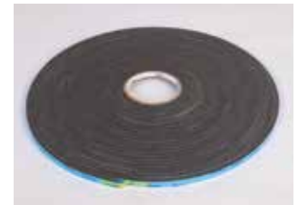
Structural Glazing Tape V2100: US made, grey urethane single & double sided adhesive. Used for when compression of tape needs to be minimal. All widths 9mm, others available upon request. Thicknesses 1.6, 3.2mm, 4.8mm, 6.4mm & 9.5mm. 24 rolls/box.
