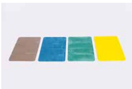
Panel Shims: Tilt-up panel construction packing shims, 150,x100mm. UV stable with 20 tonne rating. 1mm pack of 200, 2mm pack of 200, 3mm pack of 100, 5mm pack of 100, 10mm pack of 40, 15mm pack of 40 & 20mm pack of 30.
