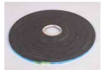
Structural Glazing Tape V2100: US made, grey urethane single & double sided adhesive. Used for when compression of tape needs to be minimal. All widths 9mm others available upon request. Thicknesses 1.6, 3.2mm, 4.8mm, 6.4mm & 9.5mm. 24 rolls/box.
