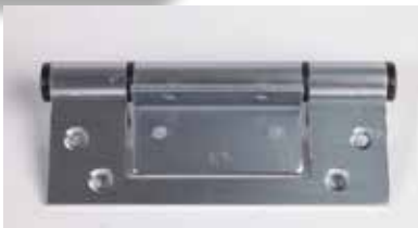
Stainless Hinge: Fast fix wrap around hinge, T6 aluminium alloy with stainless steel hinge pin and tough nylon caps and bushes.
